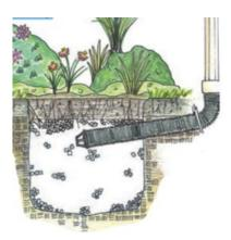
• **Dry well:** A stone-filled hole in the ground that collects runoff from gutter downspouts, roof valleys, and other areas where water concentrates and flows helps to collect roof runoff and store it until it soaks into the soil. *Image borrowed from NHDES New Hampshire Homeowner's Guide to Stormwater Management*
